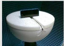
Half sphere support interface (Ø 300 mm)
