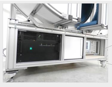
**Vector Network Analyzer** Placed in the bottom part of the frame, alongside the Integrated GigaHertz Control Unit and the PC Measurement.
