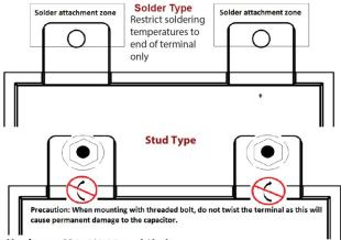
Hardware: M6≈1/4-20 stud / bolt Copper flat washer, M6 washer with 12 mm (0.472") OD
