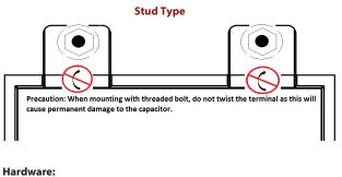
Hardware: M6≈1/4-20 stud / bolt Copper flat washer, M6 washer with 12 mm (0.472") OD
